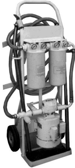
quire no tools. This unit provides optimum fluid conditioning at a lower pressure and a steady flow rate. This cannot be accomplished on many other hydraulic and lubrication systems.
